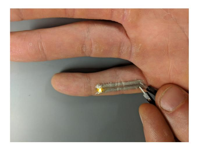
Two electronically active leads directly printed along the underside of Duke graduate student Nick Williams's pinky successfully light up an LED when a voltage is applied. Credit: Nick Williams, Duke University
