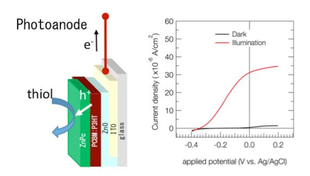
The structure of the proposed device, showing how the generated holes (h+) are used to facilitate thiol oxidation. The measured current increases dramatically under illumination and application of a slight potential. Credit: *Chemical Communications*
