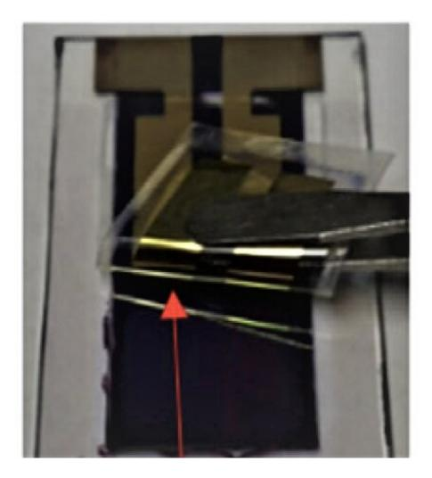
A conventional organic photovoltaic cell is removed the back electrode and processed into photoelectrochemical device that collects large volumes of electrons and holes. Credit: Kanazawa University
