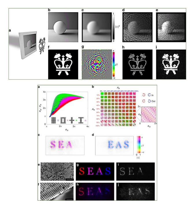
TOP: Two images encoded by a modified Gerchberg-Saxton algorithm allowing a grayscale amplitude at the metasurface plane. (a) Schematic showing the illumination of a metasurface, with an amplitude profile depicting an image of a sphere on a flat surface. The phase profile of the metasurface (not shown) encodes a holographic object (Columbia Engineering logo) at the object plane (3 mm away). (b, f) Target intensity profiles (before blurring) at the metasurface
