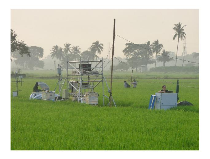
Testing of nitrogen flux measurement methods over rice in Odisha, India. Credit: Mark Sutton
