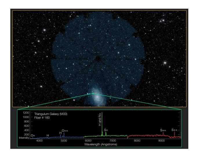
DESI's 5000 spectroscopic 'eyes' can cover an area of sky approximately 38 times larger than the full moon, as seen in this overlay of DESI's focal plane on the night sky (top). Each of the robotically controlled eyes can fix a fiber-optic
