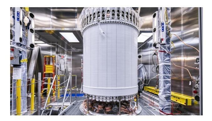
The LUX-ZEPLIN time projection chamber, the experiment's main detector, is pictured here in a clean room at the Sanford Underground Research Facility before it was wrapped up and delivered underground. Credit: Matthew Kapust/Sanford Underground Research Facility
