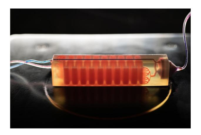
A 3D-printed cell trap developed in the laboratory of Georgia Tech Assistant Professor A. Fatih Sarioglu captures blood cells to isolate tumor cells from a blood sample. Credit: Allison Carter, Georgia Tech
