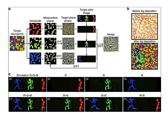
Concept demonstration of the 3D-integrated metasurfaces. (a) The flowchart of the modified Gerchberg–Saxton (GS) algorithm to generate the hologram phase. FFT is the fast Fourier transform, and IFFT is the inverse fast Fourier transform. (b) Transmission images of a random trichromatic colour microprint with 24 ×
