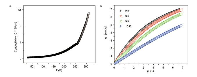
Figure 2. Electrical conductivity and magnetic properties of iodine-doped NiTAA-MOF. a) Electrical conductivity as a function of temperature. b) Magnetization increases with decreasing temperature, a typical feature of paramagnetic materials. Credit: Institute for Basic Science
