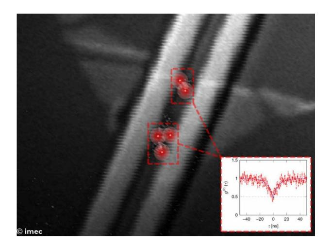
2-D monolayer on a SiN waveguide. Red shaded areas: positions of single photon emitters curve: experimental confirmation of single photon emission. Credit: IMEC
