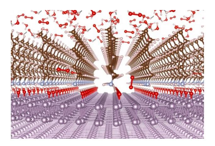
This diagram shows an edge-on view of the molecular structure of the new coating material. The thin layered material being coated is shown in violet at bottom, and the ambient air is shown as the scattered molecules of oxygen and water at the top. The dark layer in between is the protective material, which allows some oxygen (red) through, forming an oxide layer below that provides added protection. Credit: Massachusetts Institute of Technology
