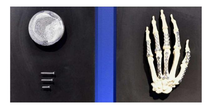
Alloys of magnesium, zinc and calcium are suitable for deployment as bioresorbable implants to fix broken bones. Credit: ETH Zurich
