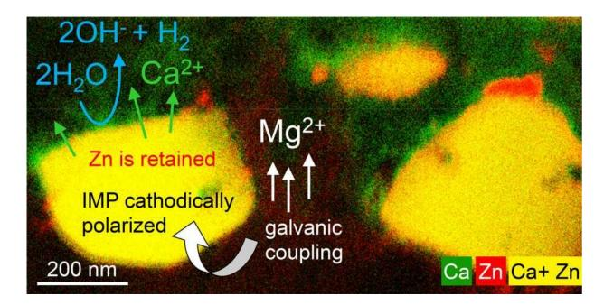
Using cutting edge technologies, ETH researchers were able to observe a previously undocumented dealloying mechanism for magnesium alloys. Credit: Laboratory of Metal Physics and Technology / ETH Zurich
