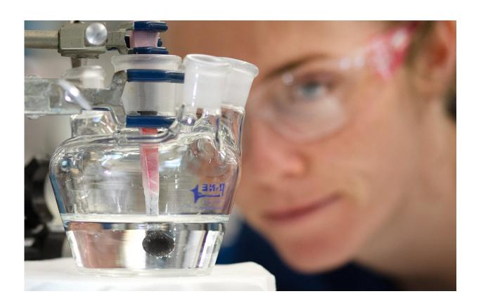
Stanford graduate student McKenzie Hubert watches a catalyst produce bubbles of hydrogen in a small, lab-scale electrolyzer. The catalyst, cobalt phosphide, is much cheaper than the platinum catalyst used today and could reduce the cost of a process for making hydrogen - an important fuel and industrial chemical - on a large scale with clean, renewable energy. Credit: Jacqueline Orrell/SLAC National Accelerator Laboratory
