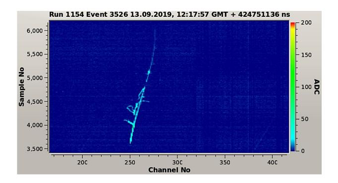
This picture shows a track made by a cosmic-ray muon observed in the dualphase ProtoDUNE detector. The ionization released by the muon track in liquid argon and by the correlated electromagnetic activity can be seen. Credit: ProtoDUNE
