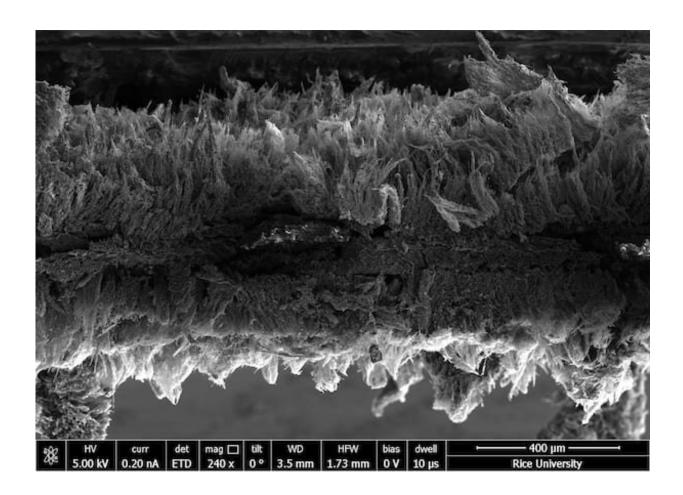
Seen in an electron microscope image, micron-scale sheets of graphene created at Rice University form a two-layer air filter that traps pathogens and then kills them with a modest burst of electricity. Credit: the Tour Group
