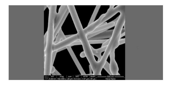
The scanning electron microscope (SEM) image shows that the Ag nanowires are completely connected after laser treatment. Credit: Li et al
