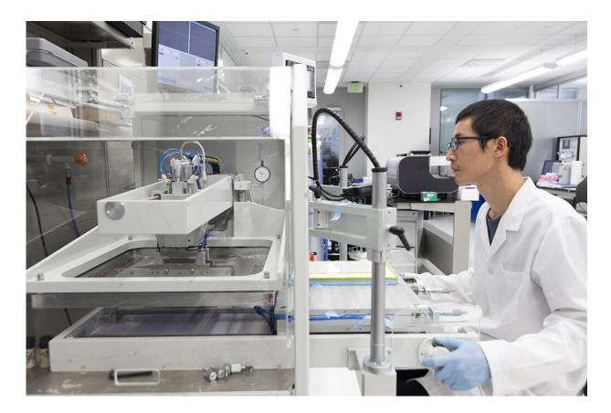
Weiwei Li manufactures the conductive, transparent nanowire sheets. Credit: KAUST
