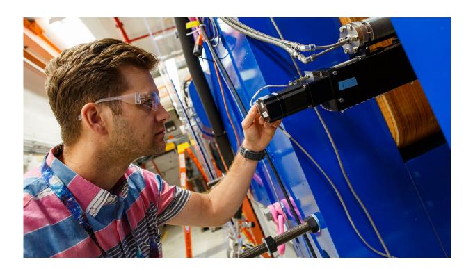
Argonne physicist Calem Hoffman works on the new Electron Beam Ion System (EBIS) at the Argonne Tandem Linac Accelerator System (ATLAS). EBIS works by increasing the charge state of ions that pass through ATLAS, allowing them to be fully accelerated. Credit: Argonne National Laboratory
