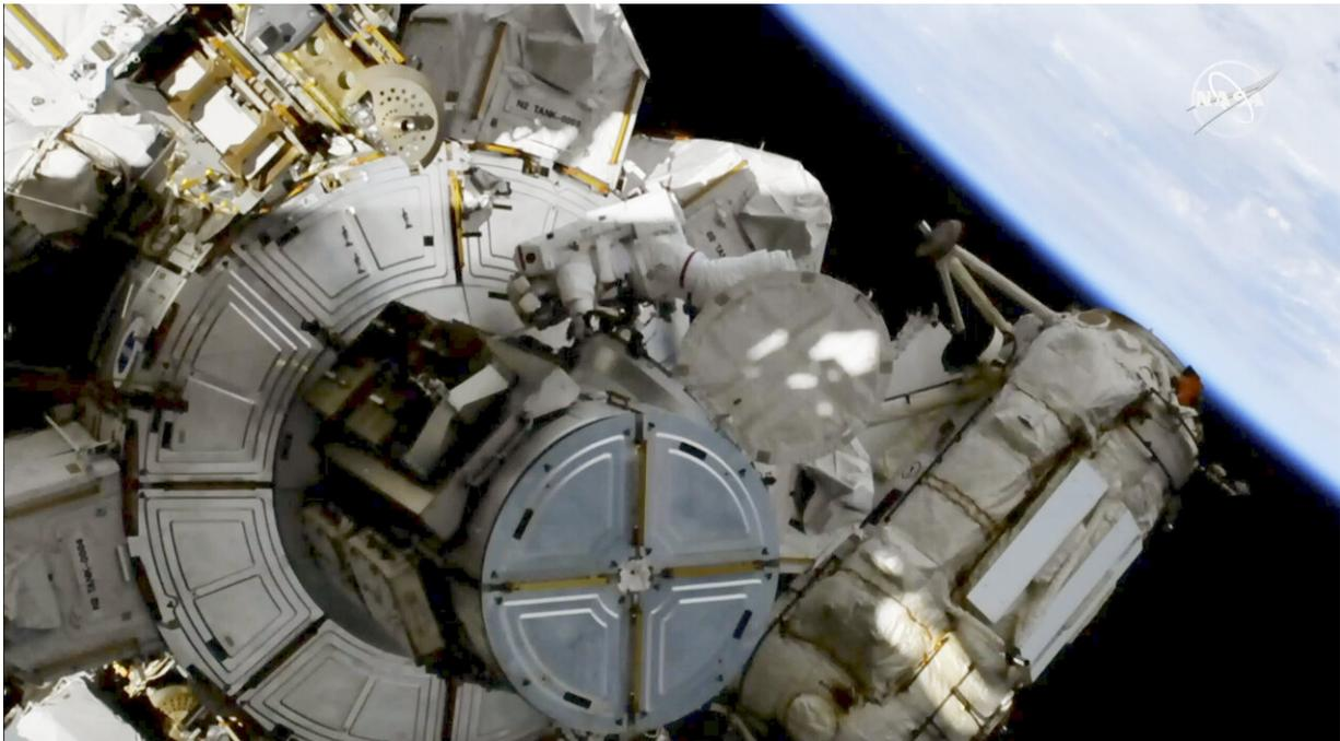
This image provided by NASA shows astronaut Andrew Morgan on a spacewalk outside the International Space Station on Friday, Oct. 11, 2019. Morgan and Christina Koch are replacing decade-old batteries in the station's solar power network with new and improved lithium-ion versions. It's the second of five spacewalks planned this month to install six new batteries that arrived via a Japanese supply ship two weeks ago (NASA via AP)
