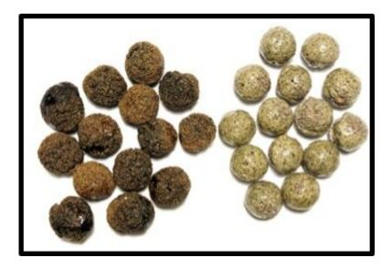
Drexel researchers are recycling coal ash, a waste product from coal power plants, to make a porous, lightweight aggregate that can be used as a concrete additive to aid the hardening process. Credit: Drexel University
