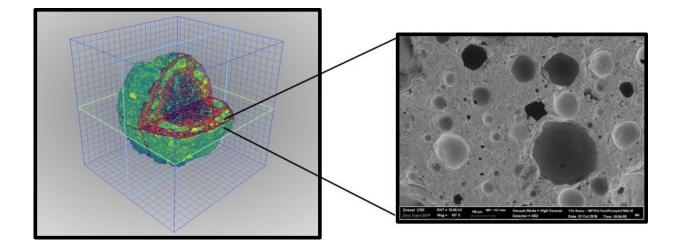
The porous lightweight aggregates created by Drexel researchers can be created in various sizes and with pore configuration tailored specifically for improving concrete curing. Credit: Drexel University
