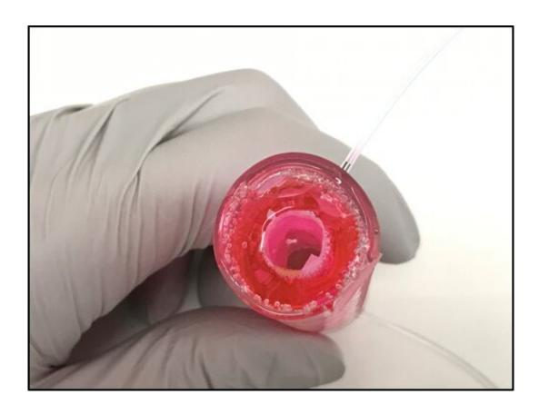
This photo shows a tubular core-shell origami gut prototype designed at the laboratory. Microbial samples are flowed through the core of the device, while the outer ring is designed to support the culture of human cells. Credit: Massachusetts Institute of Technology
