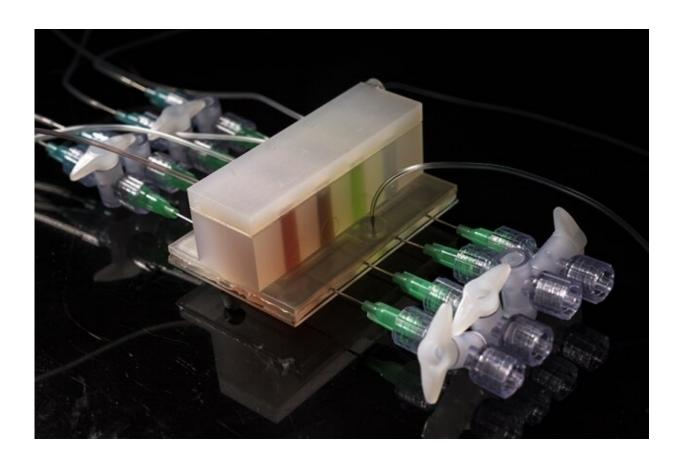
An integrated artificial gut platform developed at Lincoln Laboratory allows researchers to accurately emulate the colon, opening the way to precise testing of the human microbiome. Credit: Glen Cooper
