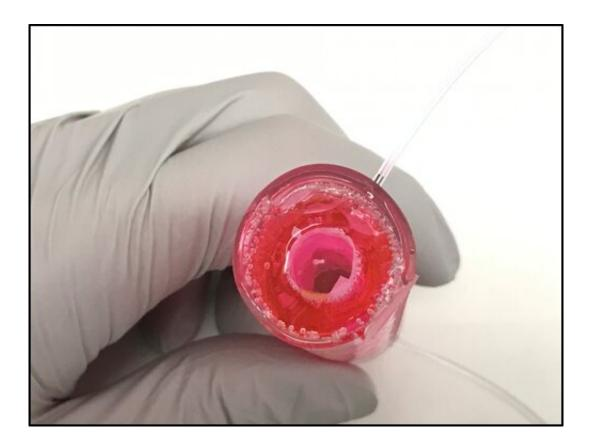
This photo shows a tubular core-shell origami gut prototype designed at the laboratory. Microbial samples are flowed through the core of the device, while the outer ring is designed to support the culture of human cells. Credit: Massachusetts Institute of Technology
