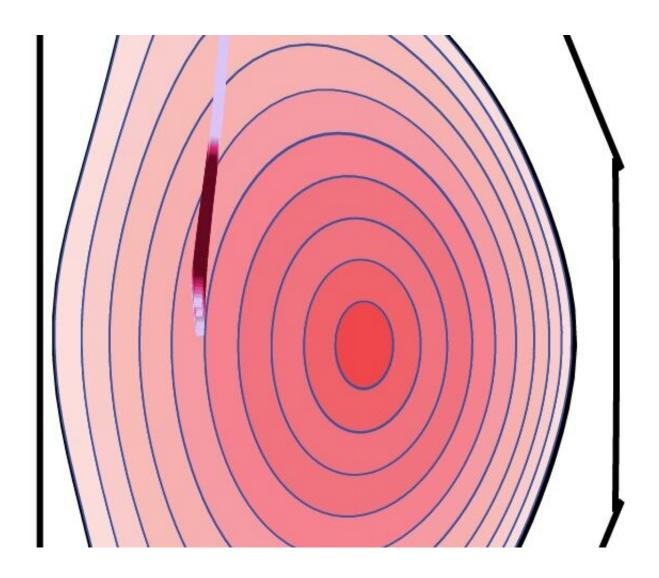
The red line shows the driven current density along the microwave trajectory in a DIII-D plasma, with the darker red showing where the larger current is driven into the plasma. This figure was modeled with the TORAY-GA ray-tracing code. Credit: Xi Chen, DIII-D National Fusion Facility.
