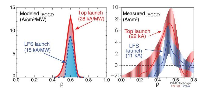
The prediction of doubling the off-axis current-drive efficiency due to more selective wave energy damping via a top-launch ECCD system has been validated by recent experiments at DIII-D. Left is prediction using the CQL3D quasi-linear Fokker-Planck code and right are measurements. Credit: Xi Chen, DIII-D National Fusion Facility
