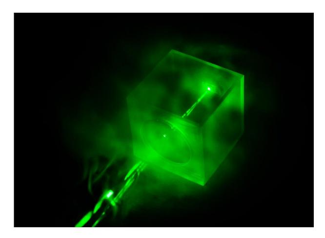
A Raman laser shining on the special chip, which traps gases and amplifies the laser signals, allowing for rapid analysis. Credit: NTU Singapore
