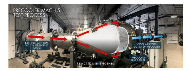
Airflow through the precooler test item in the HTX heat exchanger test programme. UK company Reaction Engines has tested its innovative precooler at airflow temperature conditions equivalent to Mach 5, or five times the speed of sound. This achievement marks a significant milestone in the ESA-supported development of its air-breathing SABRE engine, paving the way for a revolution in hypersonic flight and space access. Credit: Reaction Engines Ltd
