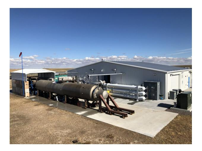
Reaction Engines' specially constructed facility at the Colorado Air and Space Port in the US, used for testing the innovative precooler of its air-breathing SABRE engine. Credit: Reaction Engines Ltd
