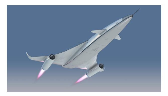
Future two-stage-to-orbit spaceplane using SABRE engines. Credit: Reaction Engines Ltd
