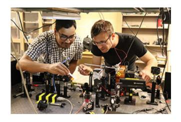
From left, Subash Kattel, a UW graduate research assistant, and Bill Rice, a UW assistant professor of physics and astronomy, use a combination of tunable, wavelength lasers and variable magnetic fields to show how spin-current-based devices can be used to measure light across a broad spectrum of wavelengths. Credit: Joshua Walker Photo
