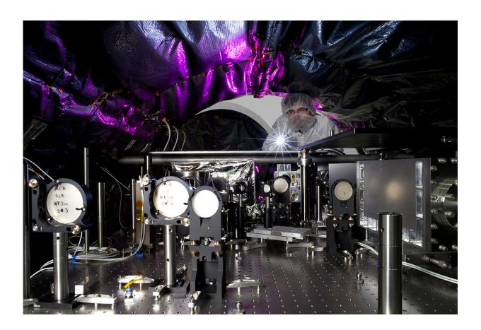
An optical engineer at NASA's Jet Propulsion Laboratory, in Pasadena, California, Camilo Mejia Prada, shines a light on the interior of a testbed for an instrument called a coronagraph that will fly aboard the WFIRST space telescope. Credit: NASA/JPL-Caltech/Matthew Luem
