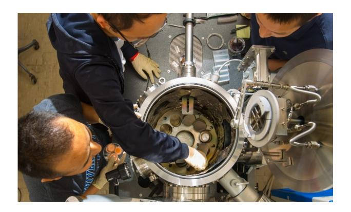
UB researchers work with a dual chamber thin film deposition system that can be used to synthesize thin film materials. In the new study, this machine was used to create europium sulfide films and tungsten trioxide, a precursor for 2D
