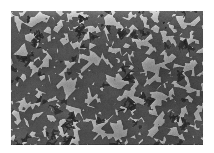
A scanning electron microscope image shows tungsten disulfide grown on a sapphire substrate (light area). The medium gray area shows monolayer tungsten disulfide and the dark area shows multilayer tungsten disulfide. After growing the tungsten disulfide on the sapphire, researchers transfer it onto europium sulfide. Credit: Chuan Zhao / University at Buffalo
