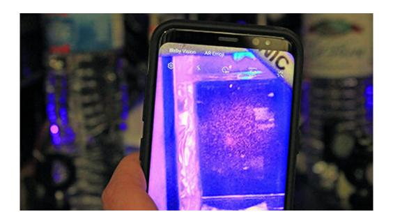
Hi-tech meets low-tech: It takes a low-quality camera to view the high-tech atomic experiments going on inside William & Mary's Ultracold Atomic, Molecular, and Optical (AMO) Physics Laboratory. This cellphone camera is able to spot a scattering of cooled atoms. Credit: Adrienne Berard
