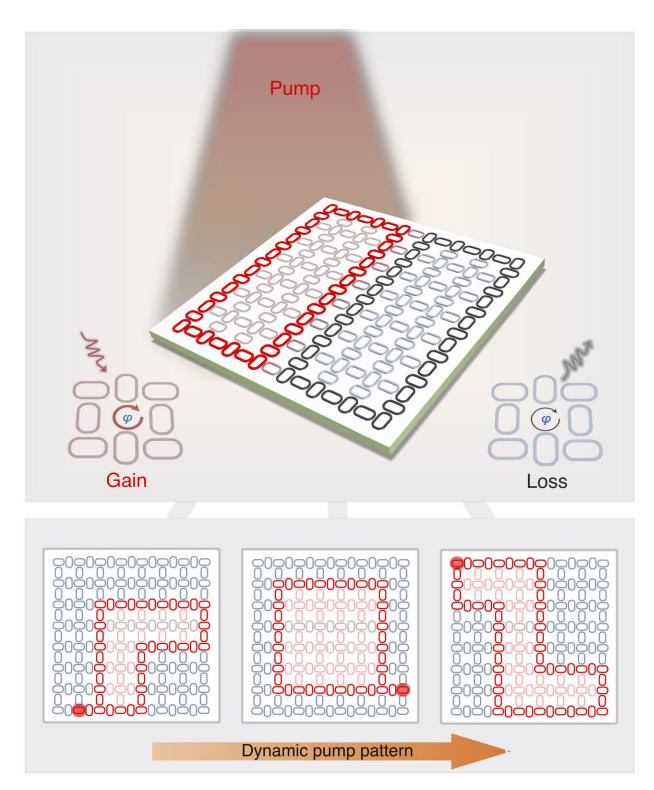
The researchers' chip features a tessellated grid of oval rings. By "pumping" individual rings with an external laser, they are able to dynamically redefine the path photons take. Credit: University of Pennsylvania
