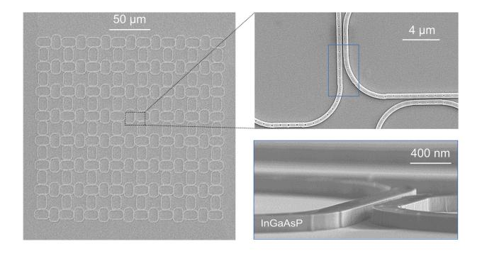
The researchers' chip features a tessellated grid of oval rings. By "pumping" individual rings with an external laser, they are able dynamically redefine the path photons take. Credit: University of Pennsylvania
