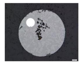
Microscope image of a sectioned micrometeorite from the Nullarbor Plain, Australia. The bright sphere is iron-nickel metal, the grey minerals are iron oxides. Credit: Angus Rogers
