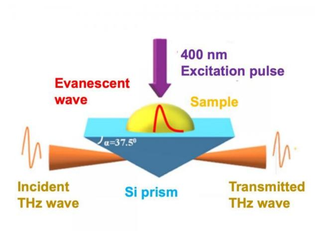
Setup for time-resolved terahertz attenuated total reflection (TR-ATR) spectroscopy. Credit: Osaka University
