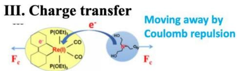
The schematic figures of the temporal evolution from I to III of the interaction between photocatalyst  $[Re(CO)_2(bpy)\{P(OEt)_3\}_2]$ + as a photocatalyst and TEOA molecules as reductants. Credit: Osaka University
