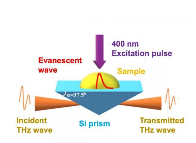
Setup for time-resolved terahertz attenuated total reflection (TR-ATR) spectroscopy. Credit: Osaka University
