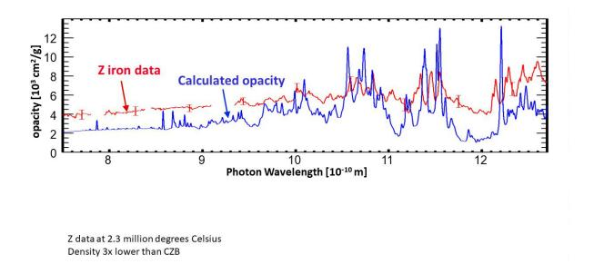
The top graph in red shows greater opacity of iron as determined experimentally by Sandia National Laboratories' Z machine. The lower graph shows the earlier theoretical calculation. Credit: Taisuke Nagayama
