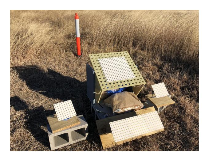
The compact Van Atta retroreflector panels designed by SwRI can be arranged in various geometric patterns, making them easy to flush mount to a surface and less susceptible to damage. Credit: Southwest Research Institute
