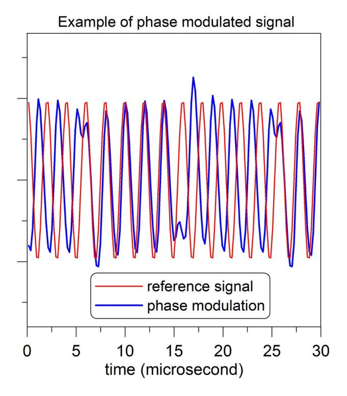
Wireless communications often use a format called phase shifting or phase modulation, in which the signals are shifted relative to one another in time. In this example, the communications signal (blue) contains periodic reversals relative to the reference signal (red). These reversals are the blips that look like
