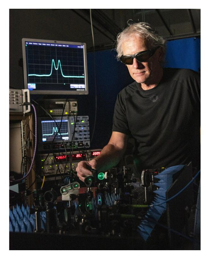
NIST researcher Chris Holloway adjusts a mirror to align a laser beam used in an atom-based receiver for digitally modulated communication signals. Credit:
