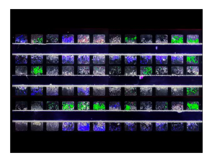
A still image pulled from UC San Diego video from three-strain co-culture experiments of E. coli. The video the image is from demonstrates autonomous cycling of the researchers' synchronized lysis circuit (SLC) that causes microbe population lysis once a threshold population density is reached. Image taken at 10X magnification. The three strains are mixed prior to loading into the microfluidic device. Strains compete until a single strain remains in each trap.
