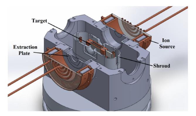
This cutaway of the high flux neutron generator shows the two chambers (bronze) where the deuterium is heated to 50,000 degrees Celsius, creating a plasma of ionized deuterium. A 100,000-volt charge at the extraction plate accelerates the ions toward the target, which contains more deuterium atoms. When two deuterium atoms fuse, they produce a neutron, which irradiates a sample placed nearby. The shroud prevents excessive heating from backstreaming electrons. Credit: Karl van Bibber, UC Berkeley
