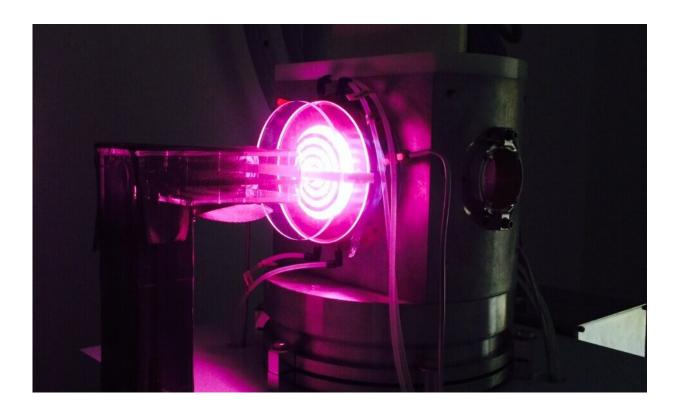
In the high flux neutron generator, UC Berkeley researchers heat up deuterium atoms in a vacuum chamber to 50,000 degrees Celsius to obtain an ionized plasma (pink glow), then accelerate the ions until they collide and fuse with other deuterium atoms implanted in the titanium cathode, releasing neutrons in the process. The spiral coil is the water-cooled radio-frequency antenna that heats the plasma, viewed through a quartz window into the vacuum chamber. Credit: Cory Waltz, LLNL
