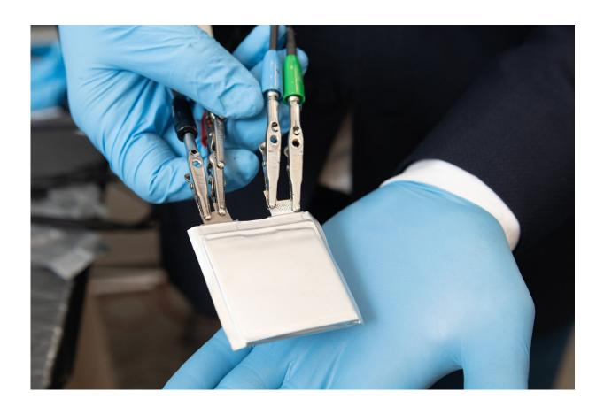
A lithium-ion battery is shown using a promising new cathode and electrolyte system that replaces expensive metals and traditional liquid electrolyte with lower cost transition metal fluorides and a solid polymer electrolyte. Credit: Allison Carter
