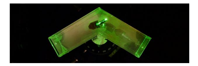
By repositioning the light source, engineers could steer the robot around slight bends. Credit: Yusen Zhao/UCLA
