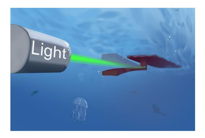
The robot's tail flapped 35 times per minute, enough to move OsciBot 1.15 times its body length per minute — about twice as fast as comparable robots that are powered by intermittent light. Credit: Yusen Zhao and Ximin He/UCLA
