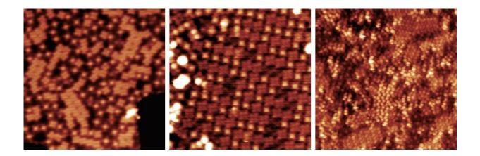
Scanning tunneling microscopy images of the organic layer at 0.6 molecule thick (left), 1.0 molecule thick (center) and 1.9 molecules thick (right). Credit: © 2019 Isshiki et al.
