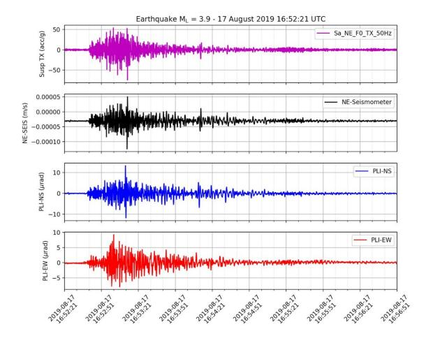
The PLI (bottom two plots) picked up the same signals as devices already installed at Virgo (top two plots) for an earthquake in Northern Italy on 17 August. Credit: Beniamino Di Girolamo/CERN
