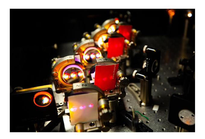
The comprehensive setup that NTU Assoc Prof Loh used, comprising a chirped mirror compressor to generate five-femtosecond laser pulses. This allows for the rapid observation of radiation damage on biological tissue. Credit: Nanyang Technological University
