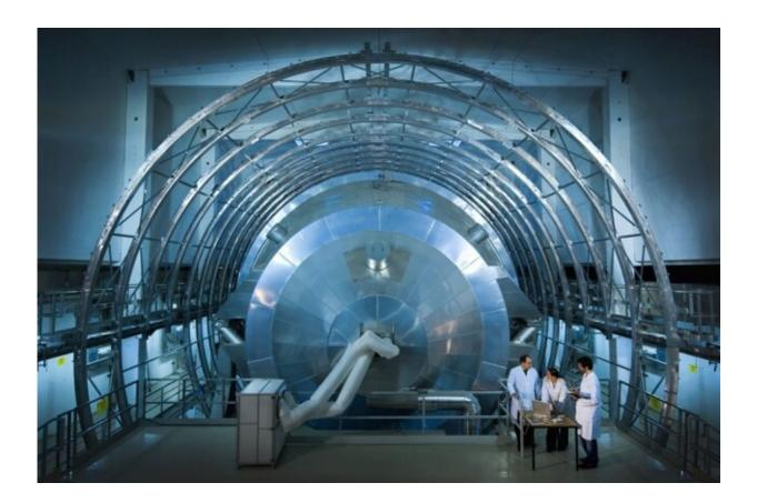
KATRIN's spectrometer, shown here, precisely measures the energy of electrons emitted in the decay of tritium, which has helped scientists come closer to pinning down the mass of the ghost-like neutrino. Credit: KATRIN Collaboration
