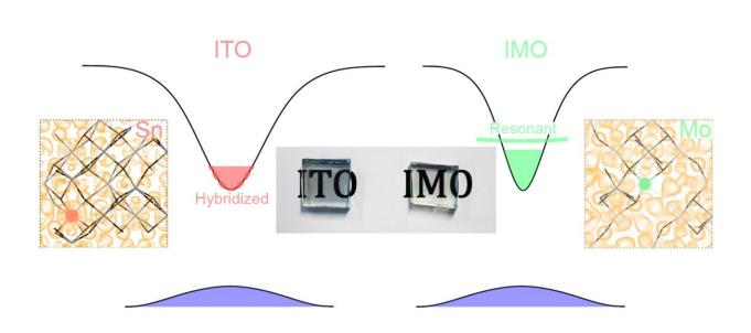
Superior transparent conducting properties of indium oxide realised by molybdenum donors resonant in the conduction band, avoiding detrimental effects of tin doping. Credit: University of Liverpool
