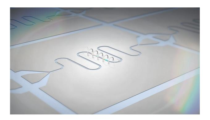
Researchers at Argonne have demonstrated an on-chip quantum circuit and realized strong coupling between a superconducting resonator and a magnetic device. The results introduce a new platform for investigating on-chip quantum magnonics and quantum information processing. Credit: Ellen Weiss / Argonne National Laboratory
