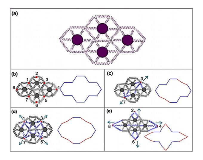
Medical implants of the future may feature reconfigurable electronic platforms that can morph in shape and size dynamically as bodies change or transform to relocate from one area to monitor another within our bodies. In *Applied Physics Letters*, a group of researchers reports a silicon honeycomb-serpentine reconfigurable electronic platform that can dynamically morph into three
