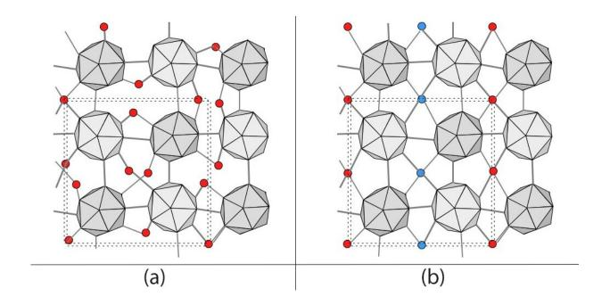
Figure 1. (a) Normal structure of  $\alpha$ -tetragonal boron. While icosahedra of boron (gray) have an ordered atomic arrangement, interstitial boron atoms (red) are randomly arranged. (b) Interstitial atoms are arranged in an ordered form in which the linear chains of interstitial atoms with different heights (red and blue) are alternately arranged. Credit: Osaka University
