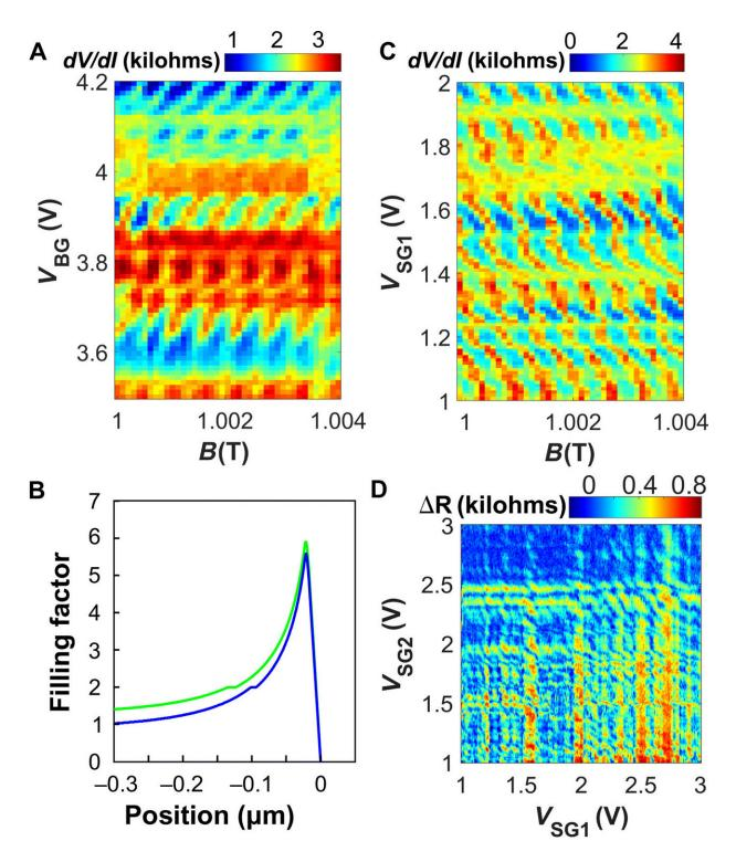
QH supercurrent interferometry. (A) dV/dI map measured at VSG1 = 2.34 V and VSG2 = 2.36 V as a function of VBG and B near 1 T. For a given gate voltage, the regions of suppressed resistance correspond to stronger supercurrent. The phase of the oscillations depends on the gate voltage, indicating that the
