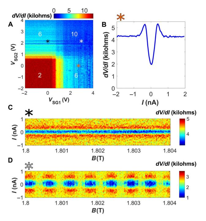
QH supercurrent and its interference patterns. (A) Differential resistance map versus VSG1,2 as in Fig. 2A but measured with 0 nA DC current bias, allowing observation of suppressed resistance due to the supercurrent. The gate voltage locations of (B) to (D) are marked by (B) an orange asterisk, (C) a black asterisk, and (D) a white asterisk. (B) dV/dI measured versus I, indicating the presence of a supercurrent on top of the quantized h/6e2 plateau. (C) Current-magnetic field
