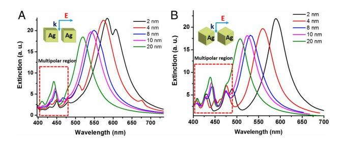
DDA calculated extinction spectra for the AgNCs in (A) FF and (B) EE orientations at varying separation distances of the dimer (2, 4, 8, 10, and 20 nm). The incident light is polarized along the interparticle axis.
