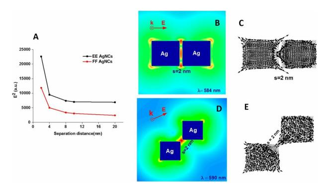
(A) Field enhancement values for the FF AgNCs and EE AgNCs at varying separation distances of the dimer (2, 4, 8, 10, and 20 nm). The wavelength of excitation was chosen based on the peak maximum within extinction spectra in Fig. 1 for each separation distance. (B–E) Field contour and polarization vector plots for the dimer of 42 nm FF AgNCs and EE AgNCs at 2 nm separation.
