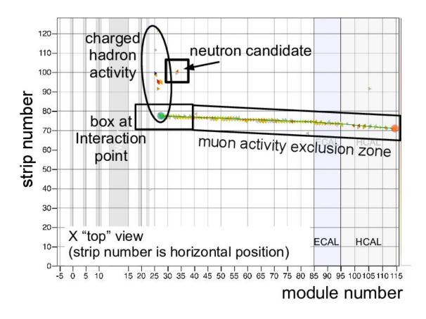
This graphic illustrates a neutrino interaction in the MINERvA detector. The rectangular box highlights the spot where a neutrino interacted inside the detector. The square box just above it highlights the appearance of a neutron resulting from the neutrino interaction. Credit: MINERvA
