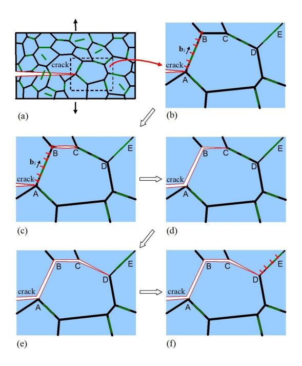
Crack propagation over grain boundaries in the composite. Graphene plates are marked by green lines. Credit: Peter the Great St.Petersburg Polytechnic University
