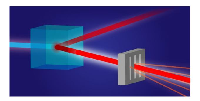
Quantum x-ray vision. A new scheme converts a high-energy x-ray photon into two lower-energy photons that are quantum correlated. Such correlations can be harnessed to boost the performance of an x-ray imaging setup. Credit: APS/Alan Stonebraker
